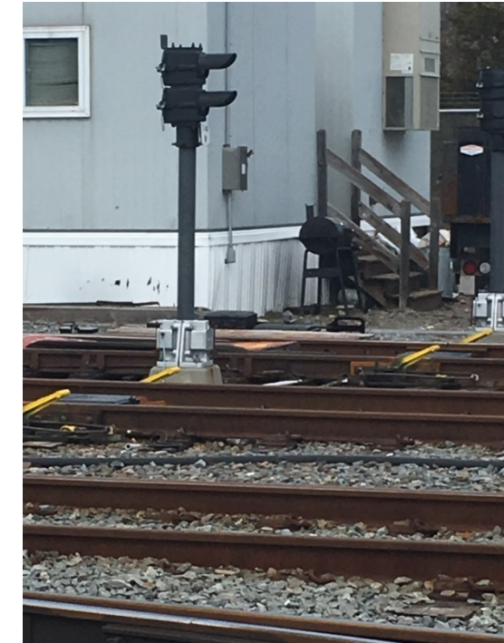
Figure 11: Blue Line Operations Signals and Power Switches entering the ROW
