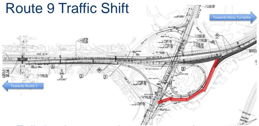
Full depth excavation, construction, and paving of the mainline and new on-ramp from Rte 9 WB to I-95 NB to occur
