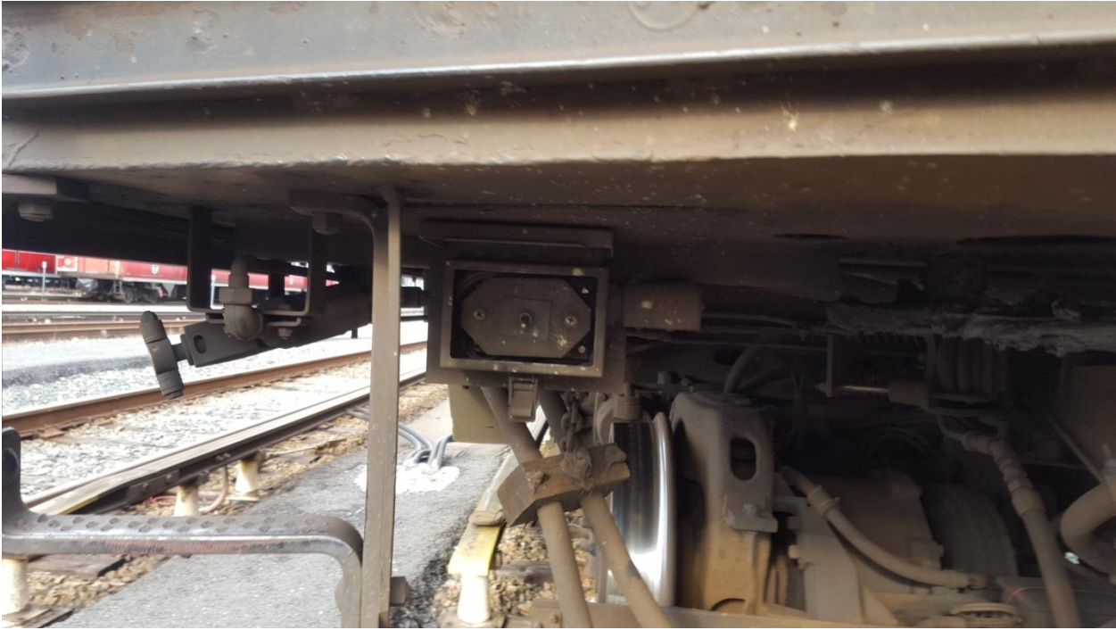
Figure 5. Red Line Emergency Bypass Switch (Outside View)
