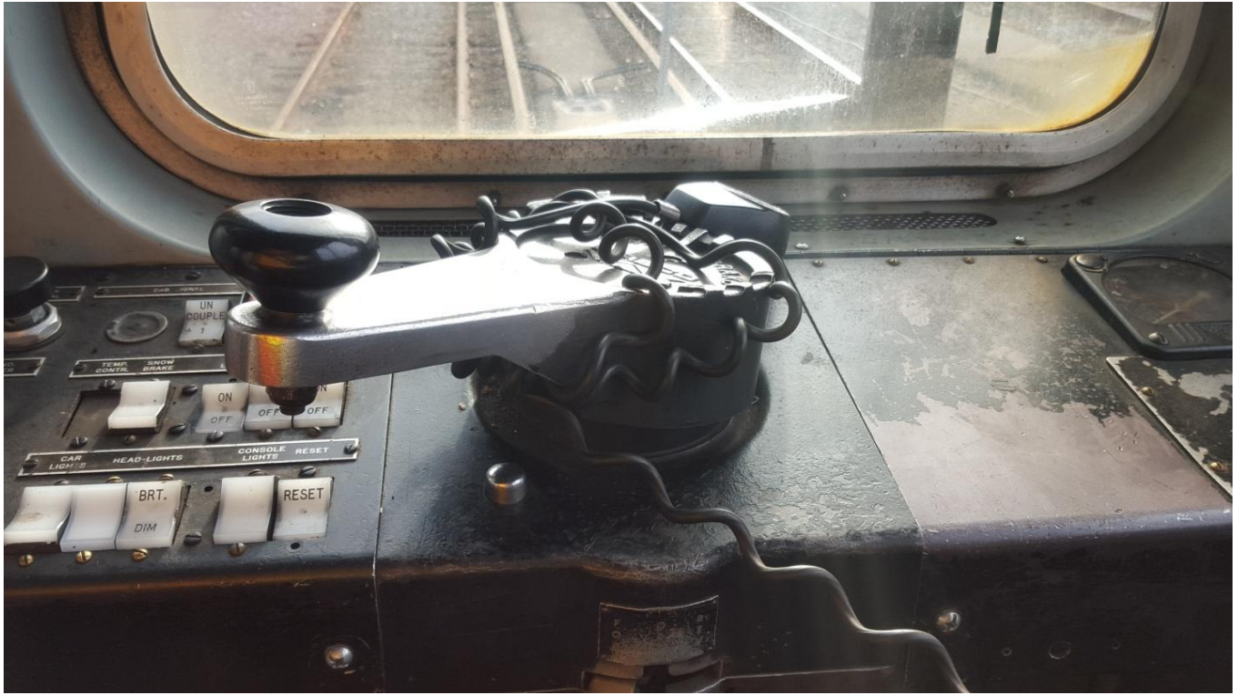
Figure 3. Cineston wrapped 2x's dead-man feature deactivated (MP view). This is a recreation based on descriptions provided.
