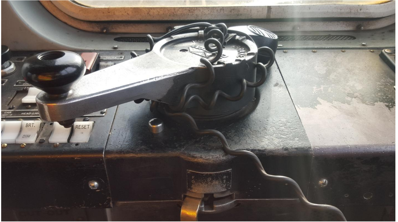
Figure 2. Cineston wrapped two times as described by responding personnel and customers with the dead-man feature activated (MP view). This is a recreation based on descriptions provided.
