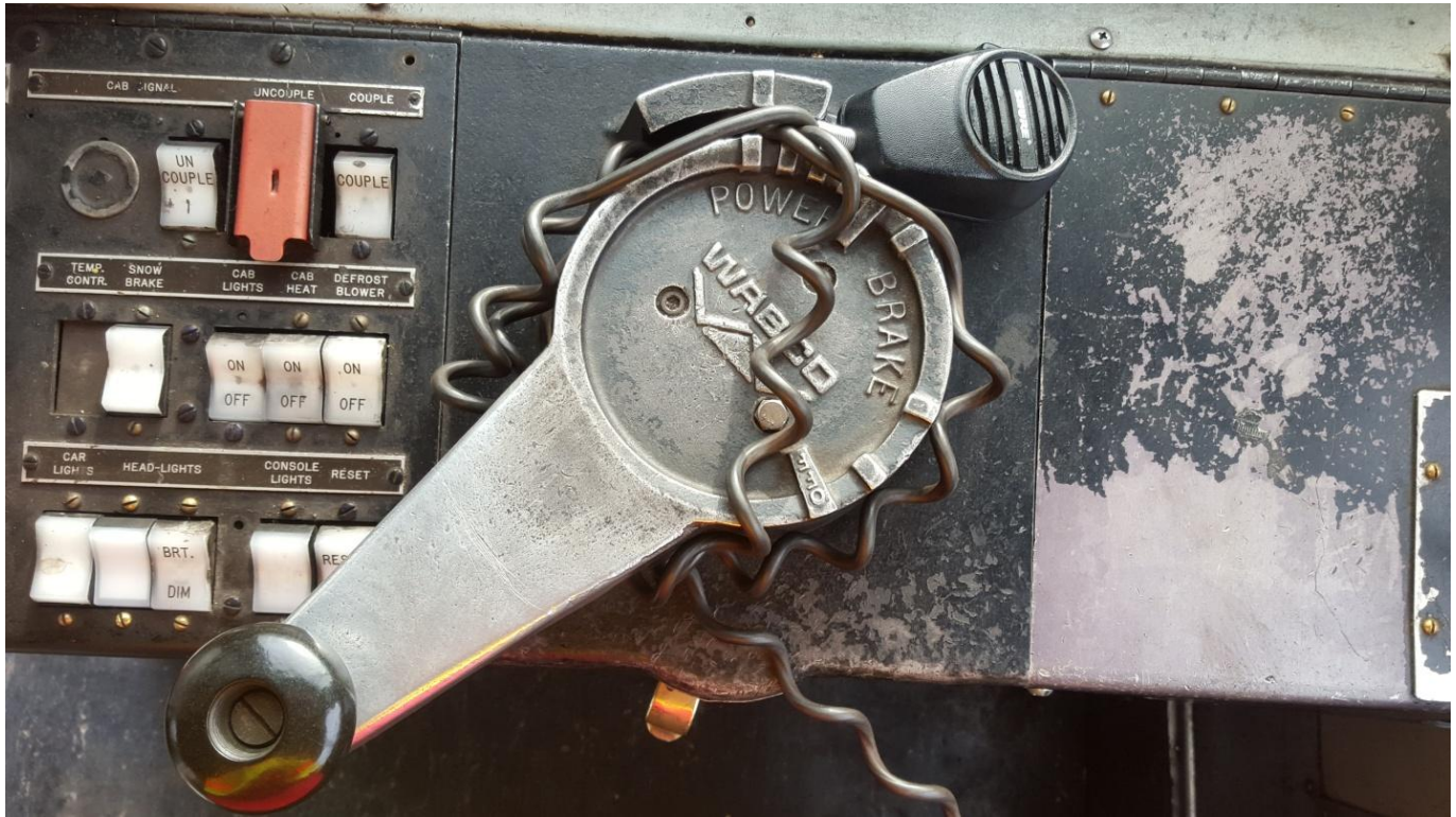
Figure 1. Cineston handle wrapped 2x's as described by responding personnel and customers with the dead-man feature activated (above view)
